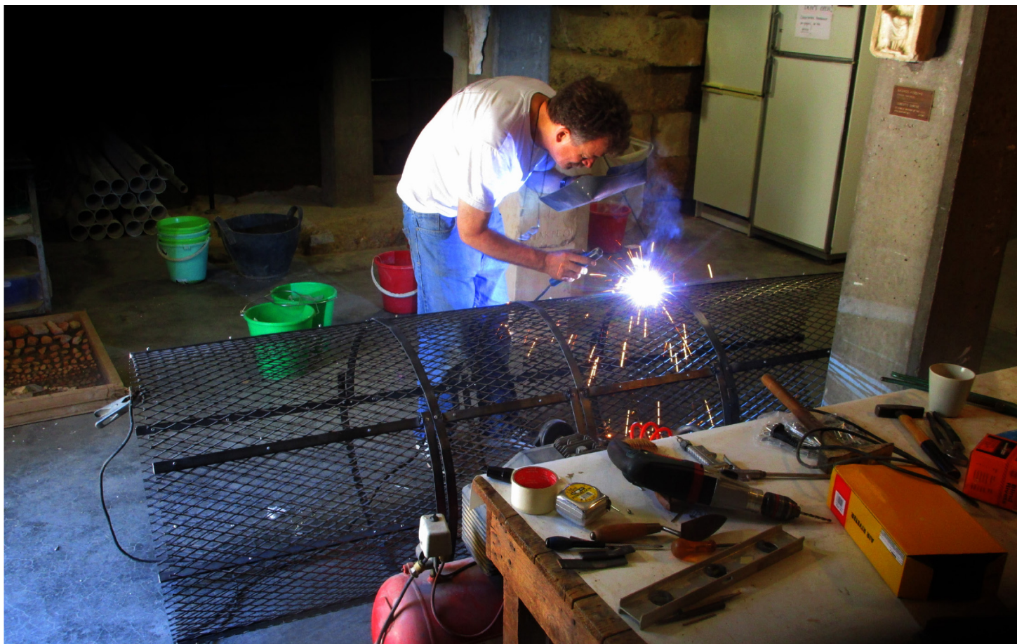
Fig. 4 Craig Mauzy finishing construction of the steel cage used for digging the well.
